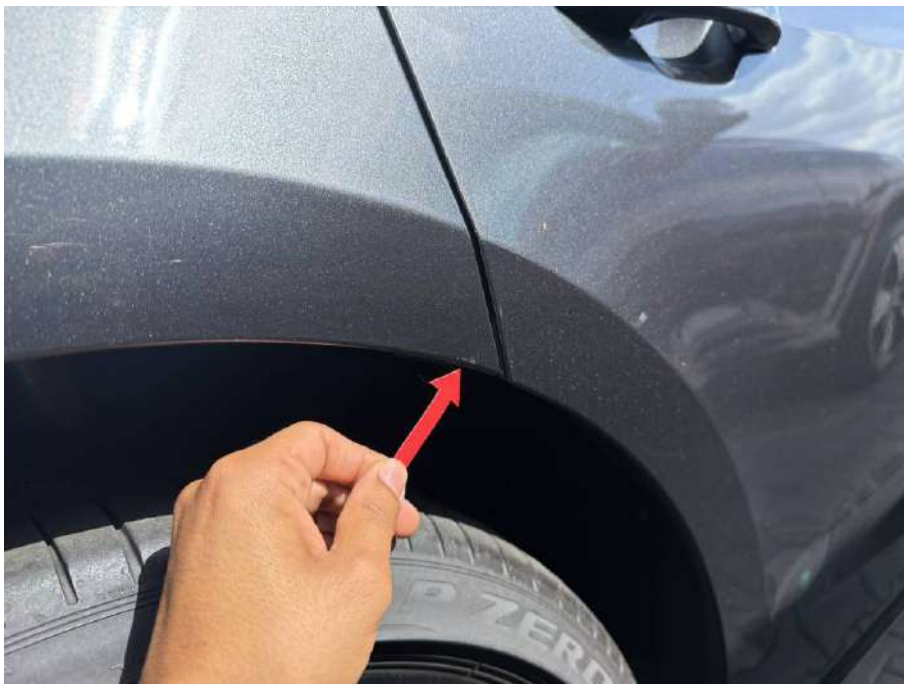
Photo 32 : Rear Right Quarter Panel - Scratch
