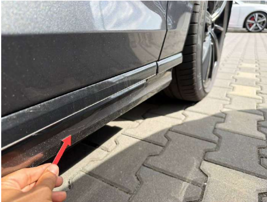
Photo 31 : Right Sill - Scratch
