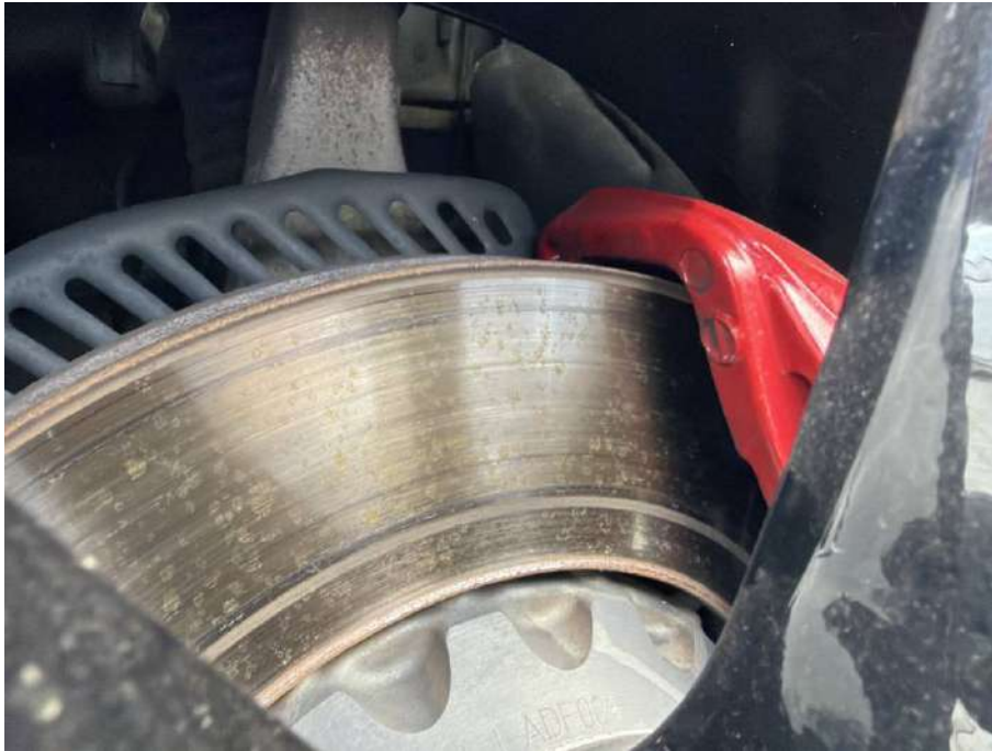
Photo 35 : Brake Discs - Close to wear limit
