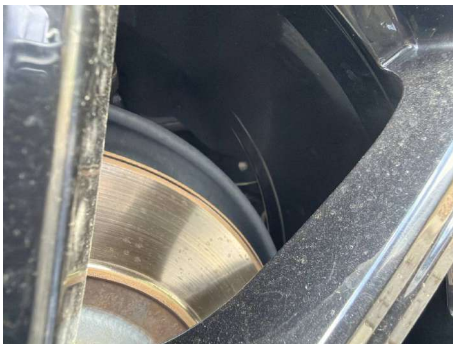
Photo 34 : Brake Discs - Close to wear limit
